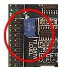
The level should be adjusted until the signal is: -3dBm, or 547mV.
