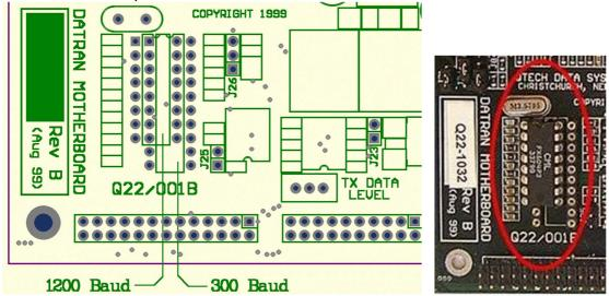
The diagram above show the locations on the left, and an installed 1200 baud modem on the right.
